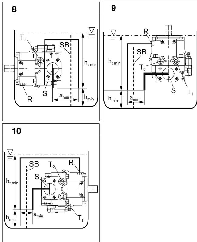
$h_{s \max} = 800 \text{ mm}$ ,  $h_{t \min} = 200 \text{ mm}$ ,  $h_{\min} = 100 \text{ mm}$ ,
