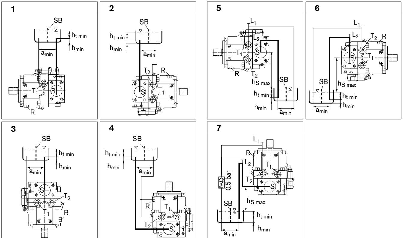
$h_{s \max} = 800 \text{ mm}$ ,  $h_{t \min} = 200 \text{ mm}$ ,  $h_{\min} = 100 \text{ mm}$ , SB = Silencer plate (baffle plate)
